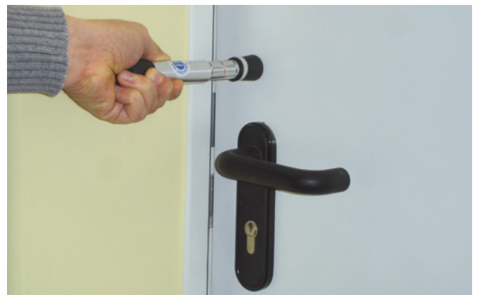
Measuring the door-opening force
